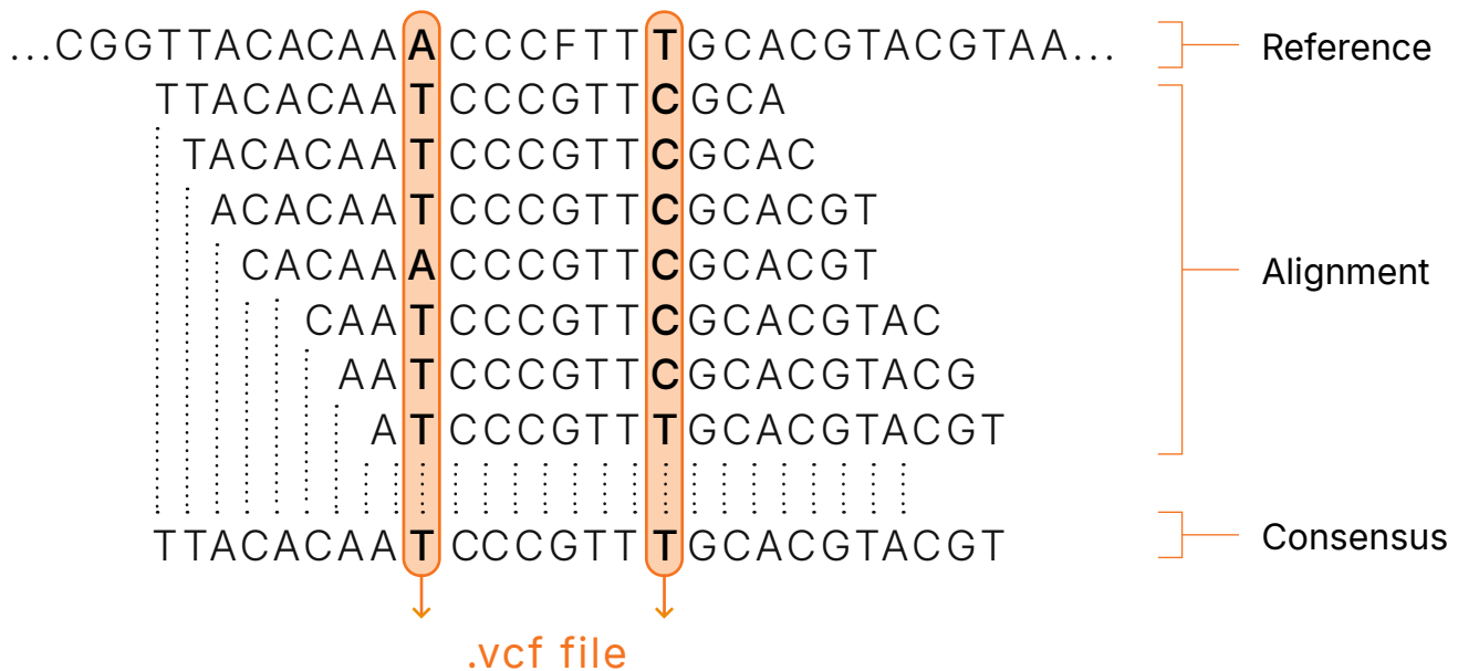
Figure 5: An example of the variant calling process, resulting in a consensus sequence.
