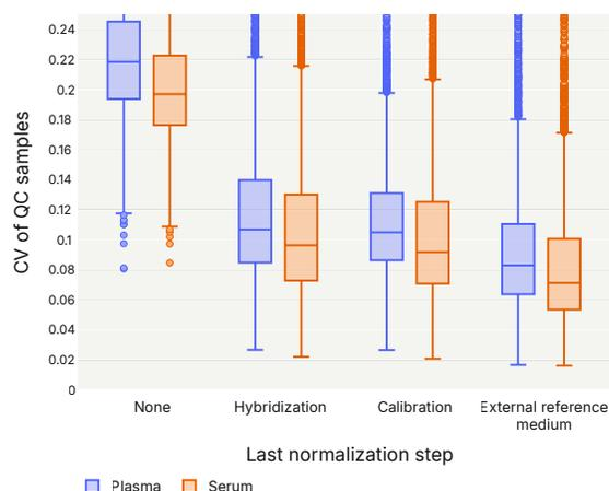
Normalization of raw assay data results in reduced intraplate coefficient of variation (CV). Data were generated using the Illumina Protein Prep 6K assay with plasma and serum QC samples. The Illumina Protein Prep 9.5K assay with median CV ~5.5%<sup>a</sup> is now available.
