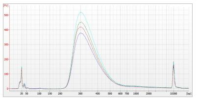
2 Use the results from the Bioanalyzer traces to determine the average size of the enriched library. Then use the following formula to convert from ng/µl to nM.
