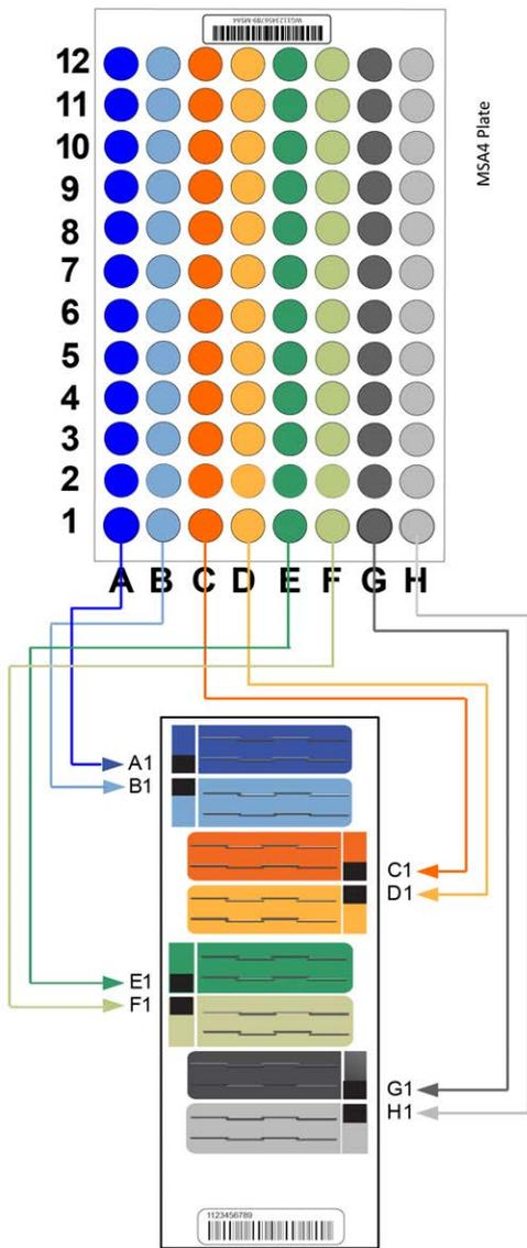
Figure 17 MSA4 Plate Layout for 12x1 BeadChip
