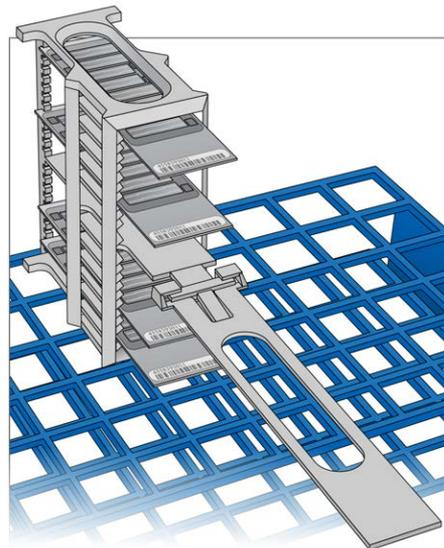
28. **[Optional]** Remove the staining rack handle to facilitate BeadChip removal:
