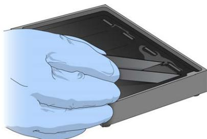
4. Place each BeadChip into a black frame, aligning the barcode with the alignment fixture ridges.
