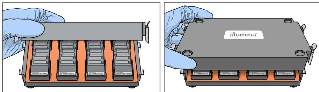
3. Close all four clamps so that the lid is secure and sits evenly on the base without any gaps. Close the clamps in the following order: top-left, bottom-right, top-right, bottom-left.
