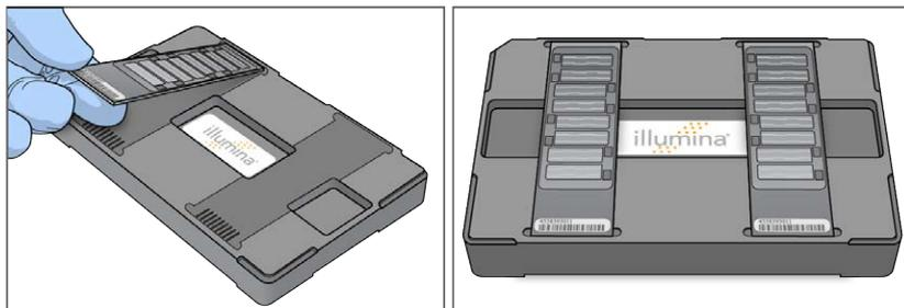
3. Stack the robot BeadChip alignment fixtures and carry them to the robot.
