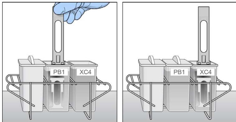
24. Slowly lift the staining rack up and down 10 times, breaking the XC4 surface. If the tops of the BeadChips touch, gently wiggle the staining rack to separate the slides.
