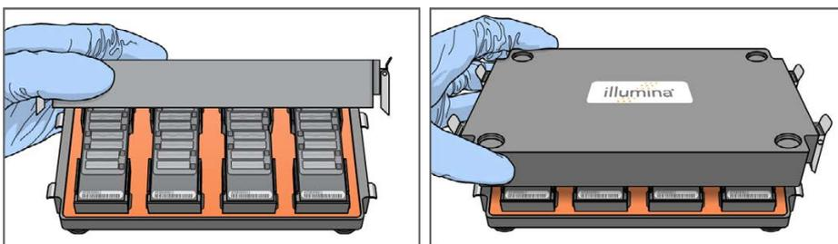
5. Close the hybridization chamber clamps in this order: top-left, bottom-right, top-right, and then bottom-left. Make sure that the lid is secure and even on the base (no gaps).
