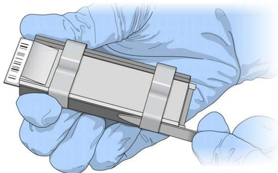
12. Lift the glass back plate straight up to remove. Set aside for cleaning after finishing this procedure. Sliding the glass along the BeadChip can damage the BeadChip.
