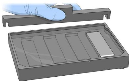
7. Place a clean glass back plate on top of each clear spacer. Position the plate reservoir at the barcode end of the BeadChip, facing inward to create a reservoir against the BeadChip surface.
