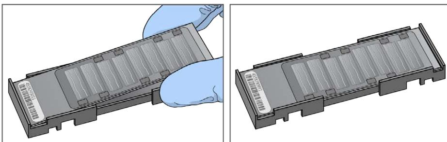
3. Make sure that hybridization chamber inserts are seated properly in the hybridization chambers.
