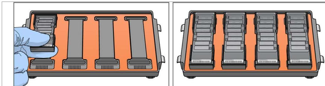
2. Place the back of the lid onto the chamber, and then slowly lower the front to avoid dislodging the inserts.
