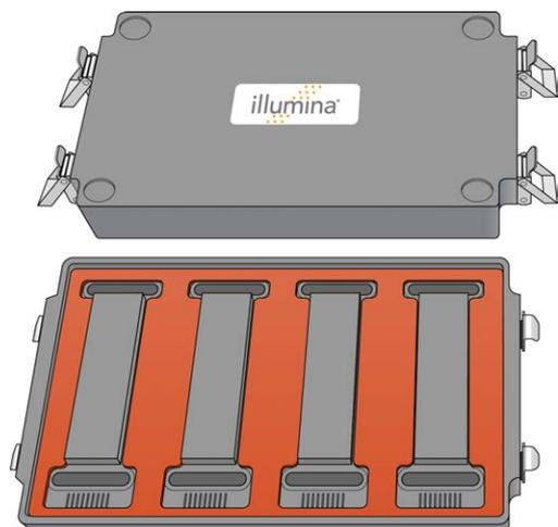
5. Add 400  $\mu$ l PB2 to the top and bottom wells of each BeadChip subchamber in the hybridization chamber.
