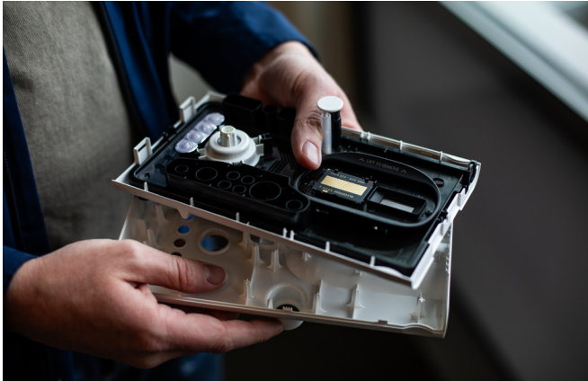
MiSeq i100 Series reagent cartridges were designed to be easily disassembled, so individual parts can be recycled appropriately.
